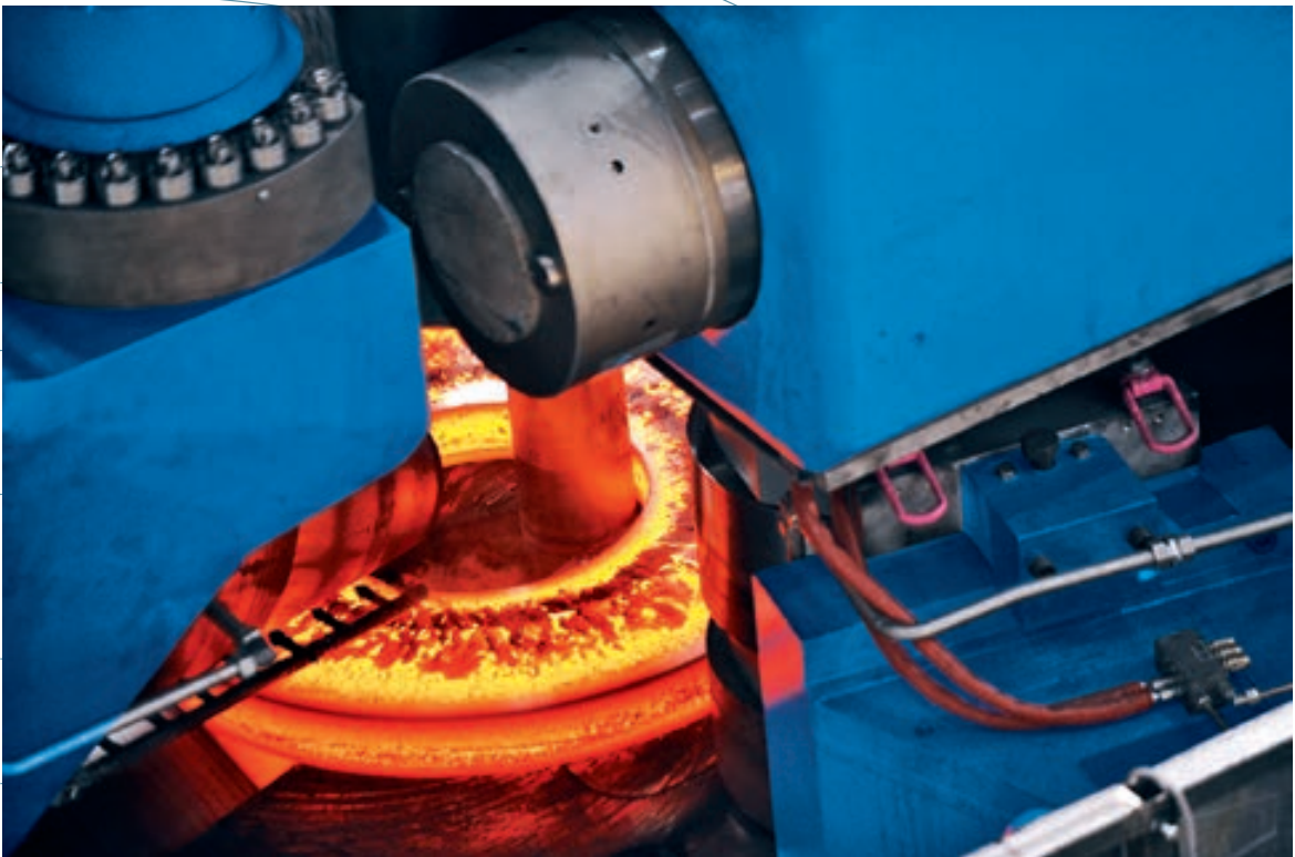
Mandrel roll inside the ring blank, axial rolls (left), and centering roll (bottom right)
