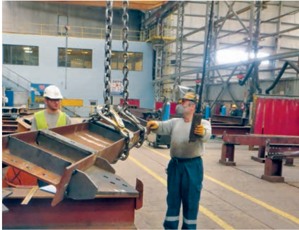
Component transport to the welding area after successful geometry inspection
