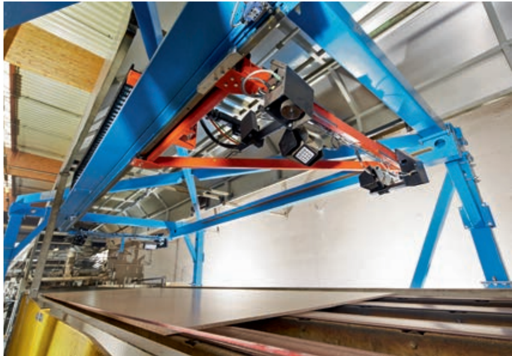
Measuring system – geometric ONLINE measuring of the board
