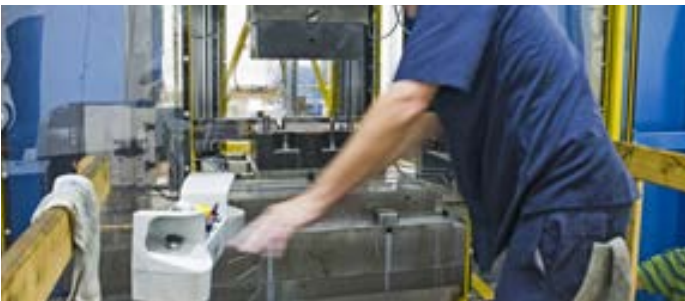
Closing the press – the hollow punches can be seen to the right and left of the blank
