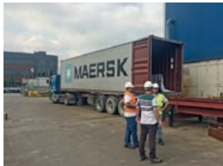
A 40ft high cube container (12 m long, 2.6 m high) ready for approx. 16 metric tons of new freight
