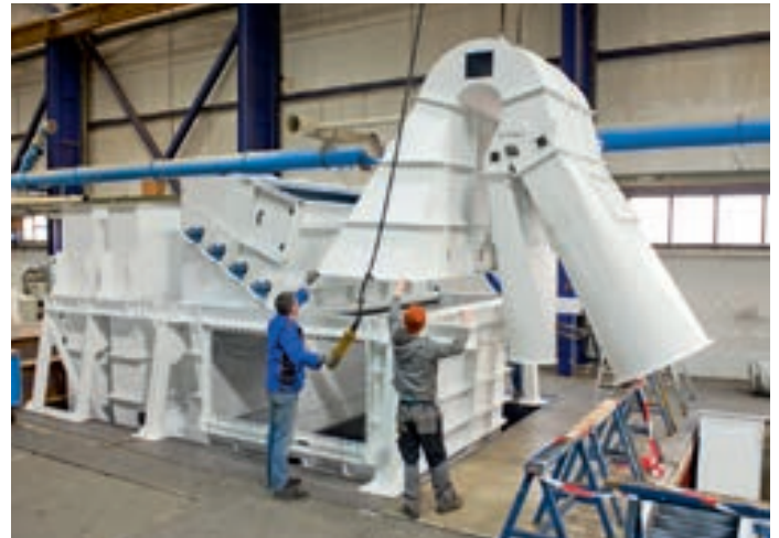
Top right: Setting the separating bend, bottom: Lifting the rotary air lock
