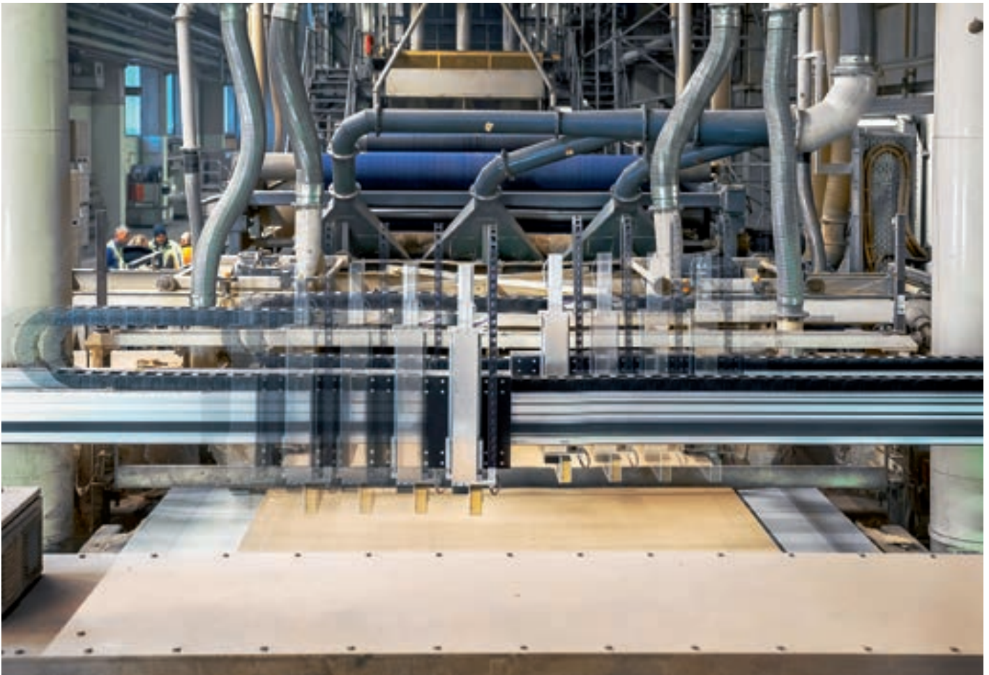
„Flying measuring head“ in operation
